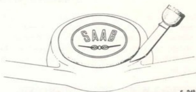
Removal of horn button, as from chassis No. 168001
