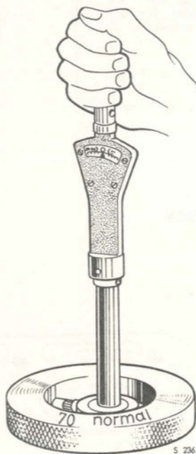
Zeroing the checking gauge
