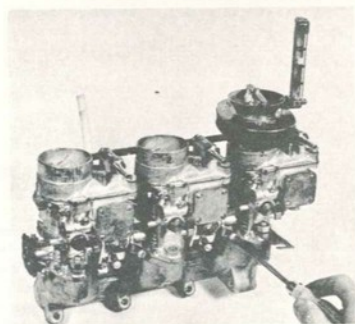
Adjusting the throttle screw with the aid of a Synchro-Test unit
